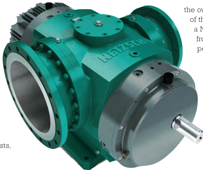
The 4NS offers a maximum flow rate of 792,500 gallons per hour and is suitable for highly viscous media with up to 200,000 cSt. At the same time, the pump has a highly robust design, from the contact free screws to the physical separated synchronization gearbox.
