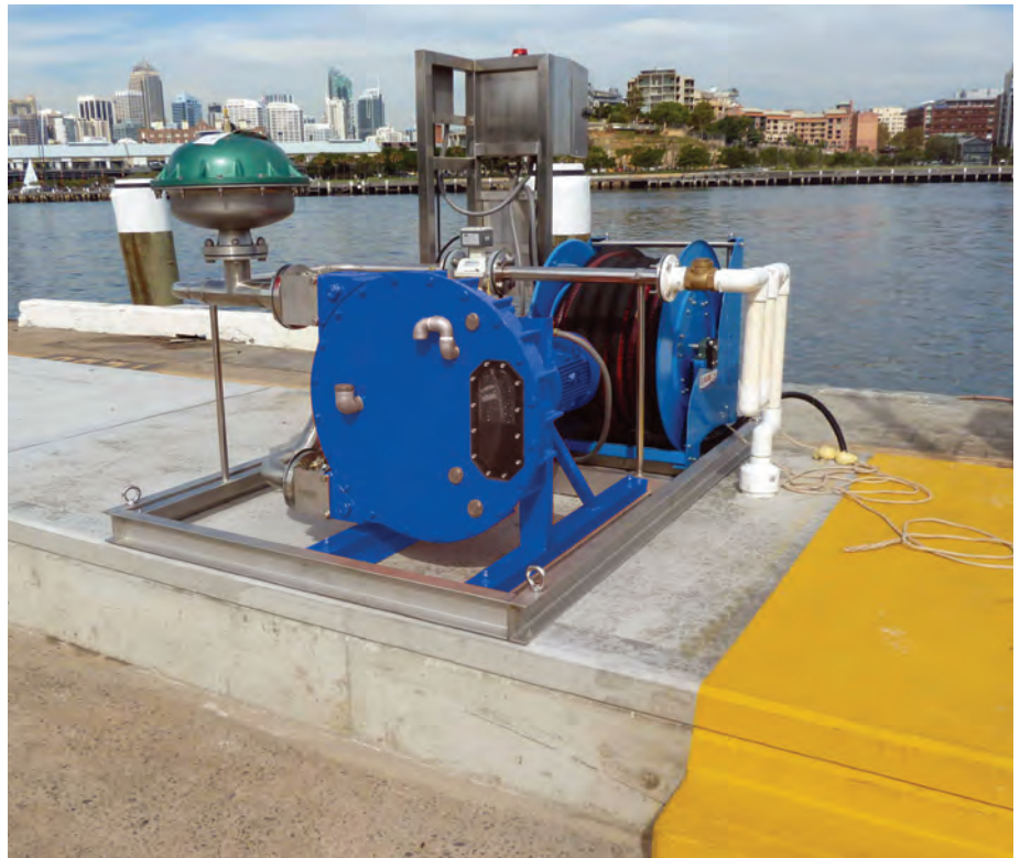
Peristaltic pumps can transfer solids and soft particles, as well as handle water-like viscosities as high as 352,000 cSt (70,000 SSU), making them suitable for industrial wastewater and municipal water treatment facilities.
