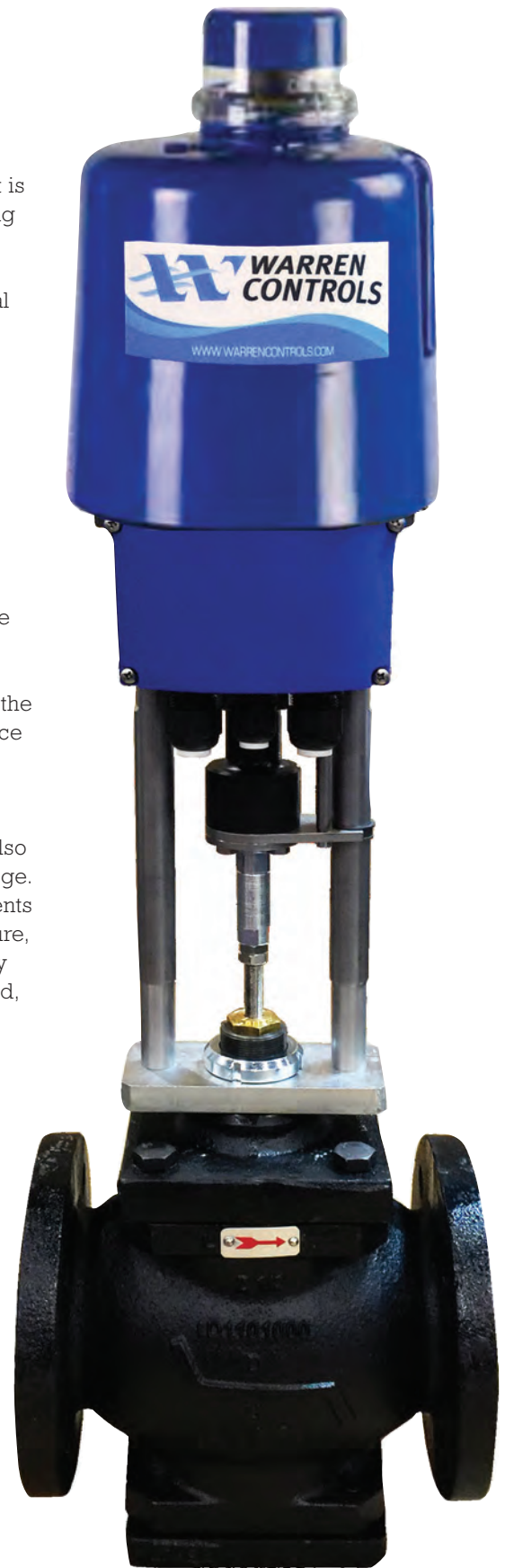
A globe valve with an electric actuator, such as the Warren Controls ILEA 5800E Series, provides a large turndown ratio and precise modulating control for steam PRV applications.
