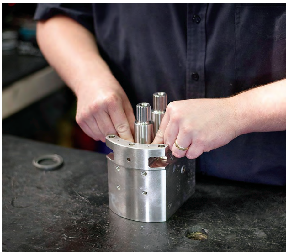
A gear pump with a clean or simplified design makes maintenance much easier for sanitary operations.
