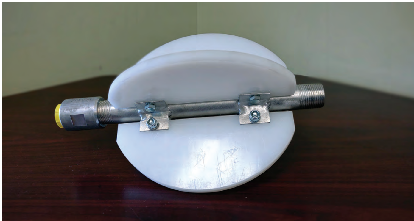
The new skid design uses a lightweight aluminum pipe core with protruding plastic fins to provide nozzle stability without the weight of heavier steel skids.
