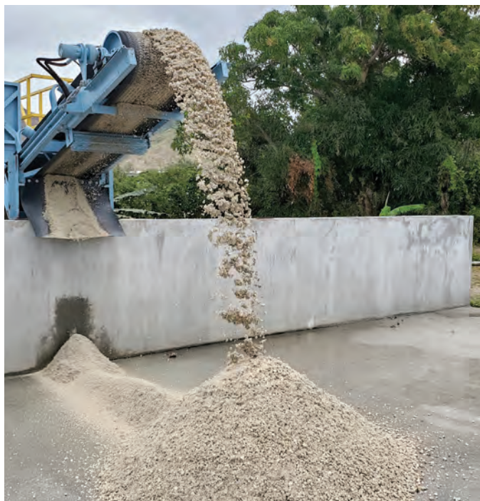
With the sophisticated systems available today, plants can now complete washout and reclaim any leftover concrete materials faster and more profitably than ever before.
