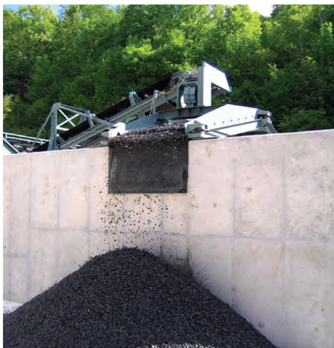
Expedited reclamation process can eliminate the need for pits, ponds, and multiple handling while providing total recovery of sand, aggregate, and cement.
