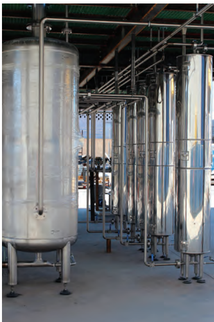
The evaporator crystallizer includes nineteen tanks and fifteen heat exchangers.
