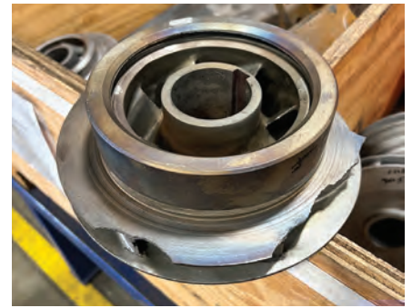
The pump in question was a between-bearing, six-stage type working with propylene carbonate, with damage to all the stationary and rotating elements contained within.
