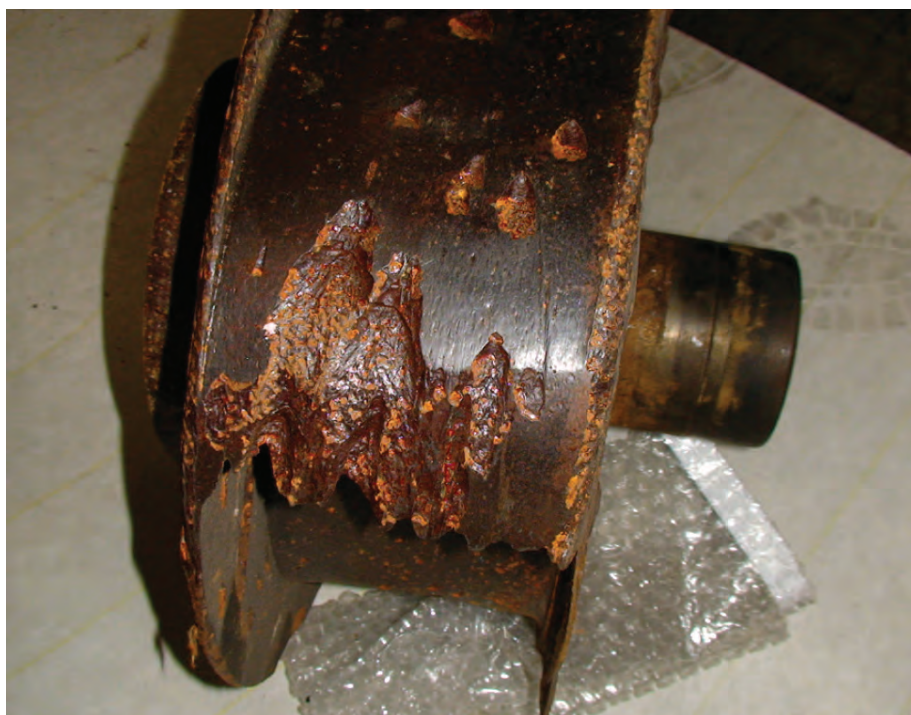
Figure 1: Furrowing that is typical of erosion.
