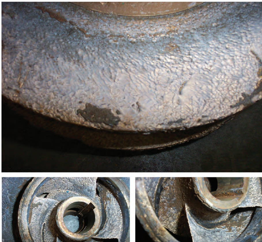
Figure 2: Corrosion damage is indicated when all exposed surfaces are affected.
