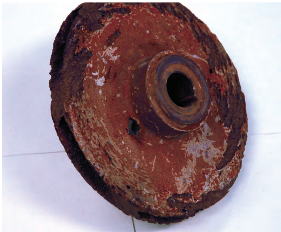
Figure 4: Cavitation where leached zinc leaves reddish-colored copper from bronze alloy.
