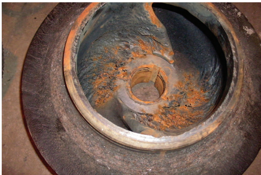
Figure 3: Cavitation damage that is limited to the suction area.
