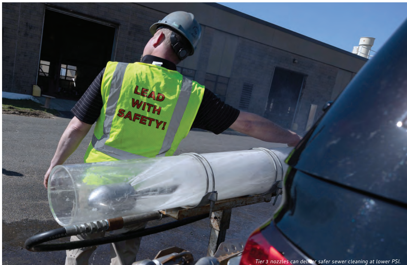
Tier 3 nozzles can deliver safer sewer cleaning at lower PSI.
