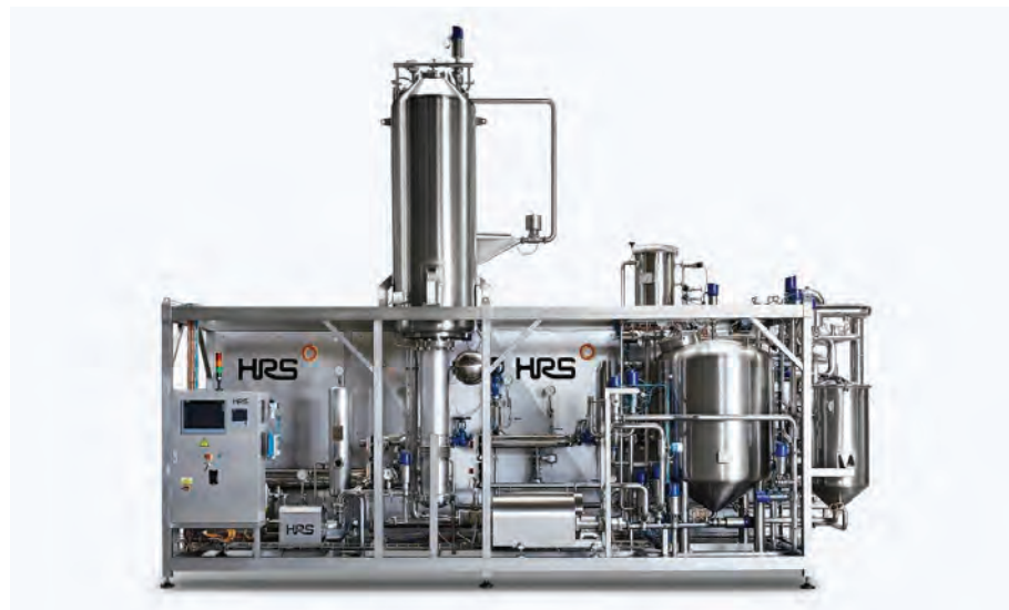
The UHT system supplied by HRS includes Direct Steam Injection (DSI) and a MI Series heat exchanger.
