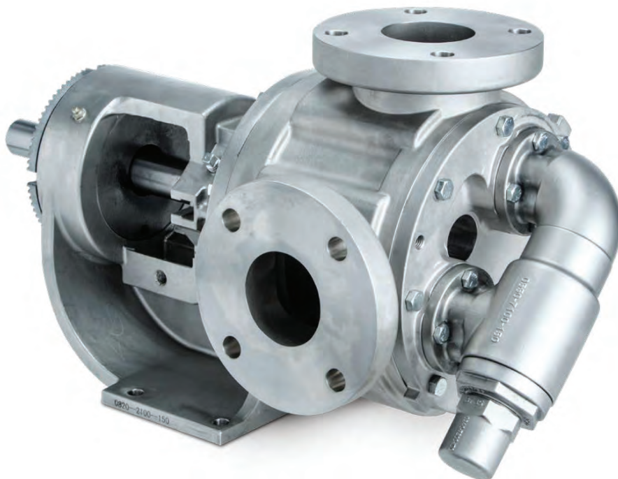
Blackmer® G Series internal gear pumps feature a jacketed cast-iron body, ANSI flanges, bronze or carbon-graphite bushings, and carbon-graphite packing or Buna-N mechanical seal.
