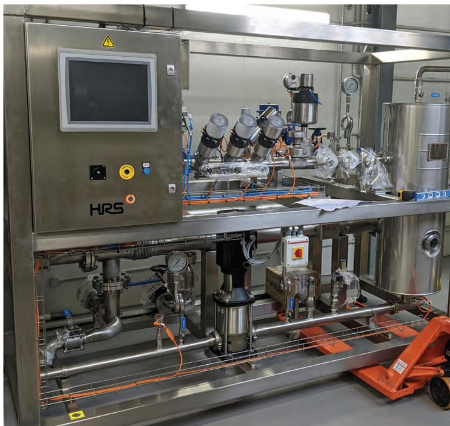
The HRS unit utilizes two K Series multi-pass corrugated tube heat exchangers to maintain solvent temperature as required.
