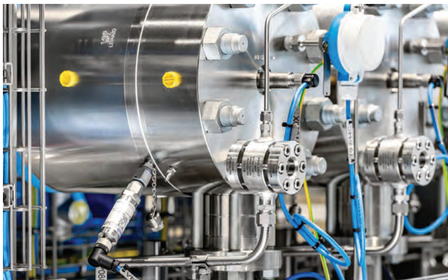
The measured values come from a structure-borne sound transmitter located on the pump body, a pressure transmitter connected to a pressure measuring bore, and a rotary encoder adapted either directly via the crank shaft or the engine. Here you can see the pressure transmitter.
