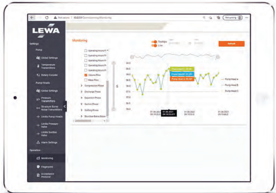
Thanks to the structure-borne sound characteristics, wear and tear on valves can even be detected before it becomes measurable in the flow rate of the system.
