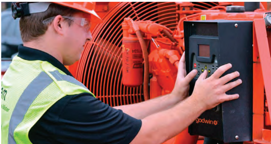
The Godwin PrimeGuard controller provides greater visibility and peace of mind by connecting with a SCADA system, registering when the backup pump is running.
