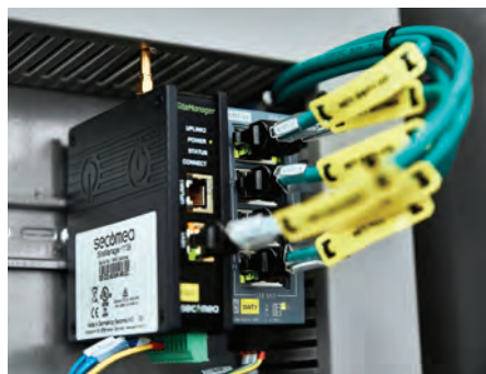
HRS systems can be connected to the Internet of Things (IoT) via ethernet or 4G SIM.
