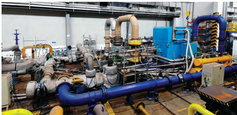
String testing of one of the feedwater pumps at Sulzer's manufacturing plant in Suzhou.
