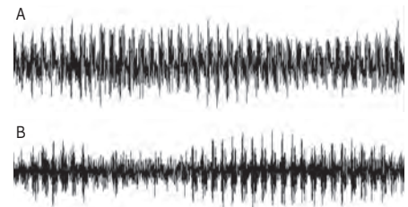
Figure 4: Baseline vs. rub vibration waveform for 3,000 RPMs.
