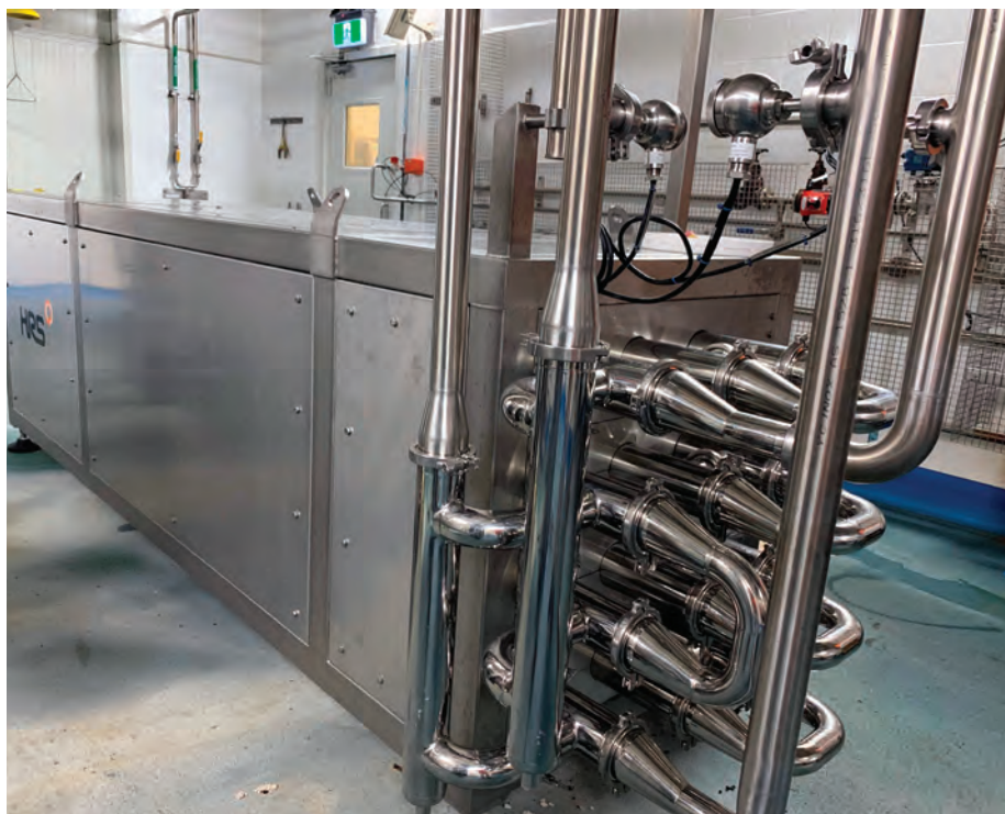
The completed thermalizer raises the temperature of the product prior to the final heater.
