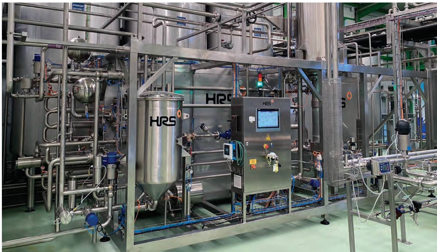
The new HRS DSI Series uses direct steam injection to increase the speed of sterilizing products such as oat milk.
