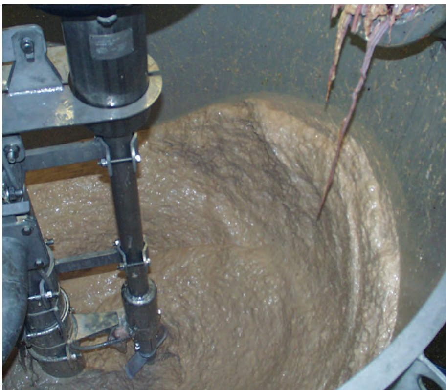
Landia mixers simultaneously mix and aerate acidic, screened poultry plant effluent.
