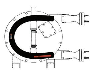
reinforcements. The smooth precision ground cover, and concentric wall, ensures optimum performance and consistent flows. Tubes of these hoses can be constructed of Natural Rubber, for abrasion resistant
