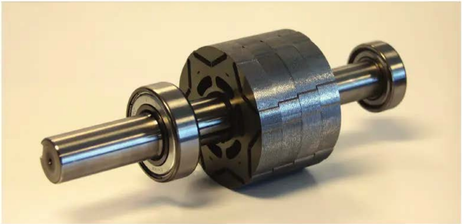
Internal permanent magnet (IPM) rotor core with skewed mounting to prevent cogging.
