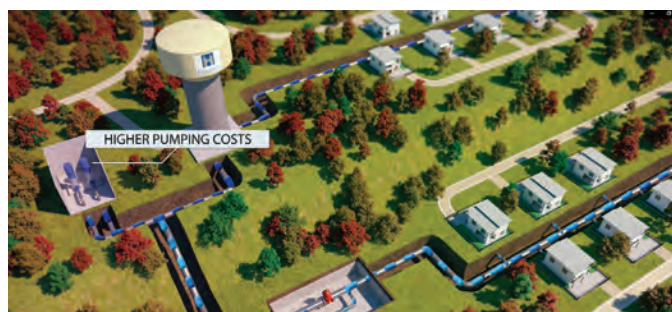
The 3/4-inch bypass line eliminates stagnant water but (1) increases pumping costs, (2) increases main breaks, (3) instigates in-chamber "mini-breaks."
