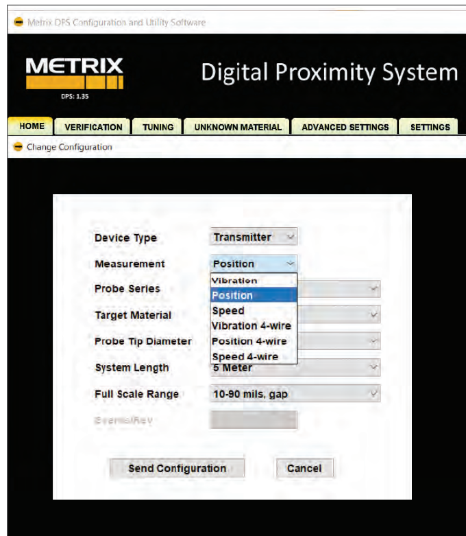
Figure 7: User interface of Metrix DPS configuration and utility software.
