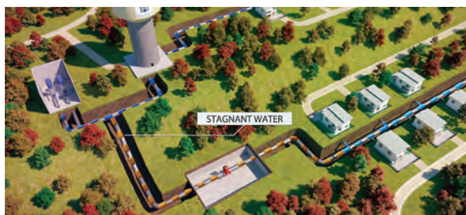
Normally-closed zone boundary valve creates two dead ends; stagnant water results.
