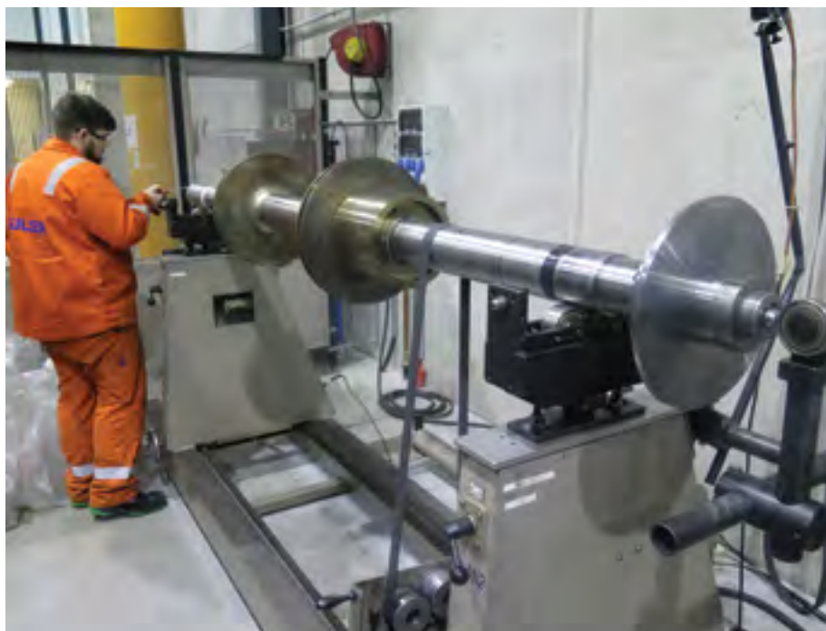
Setting up the de-staged rotor from the main pump for balancing before reassembly.
