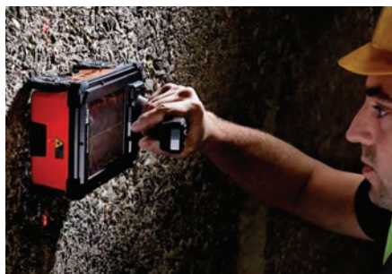
The Palm XT gives GSSI StructureScan Mini users a handheld miniaturized GPR antenna for enhanced access to tightly spaced areas.
