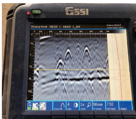
GSSI's easy-to-read visualization allowed GPRS to create drawings with locations and depths of obstacles.
