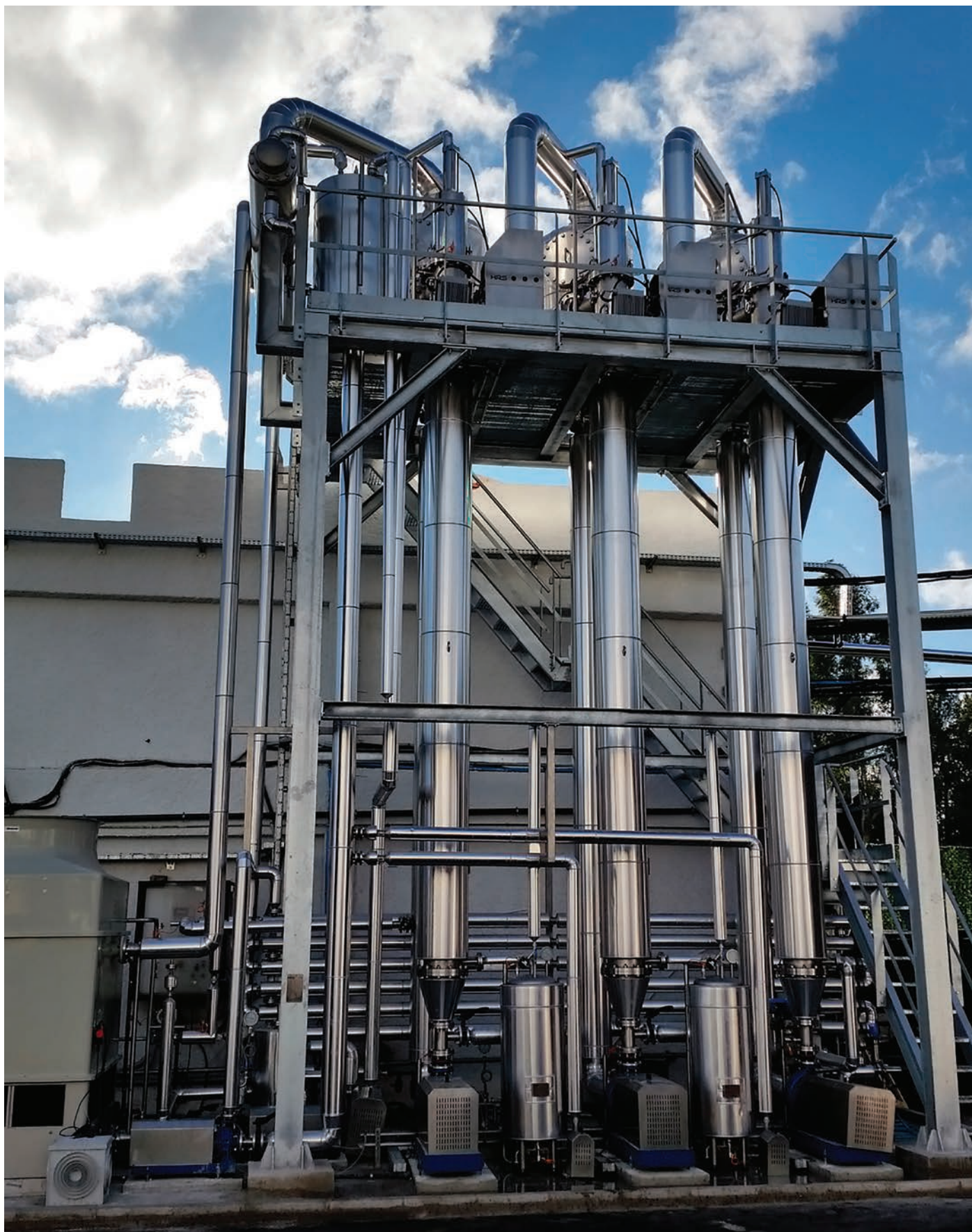
HRS Unicus Series scraped-surface evaporators are used to maintain thermal efficiency and remove fouling during evaporation in ZLD installations.
