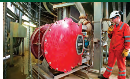
Bredel hose pumps have a corrosion-resistant enclosure which suits arduous mining environments.
