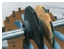
These two impellers operated for 18 months in salt water. The Simsite® Impeller is unaffected by corrosion!
